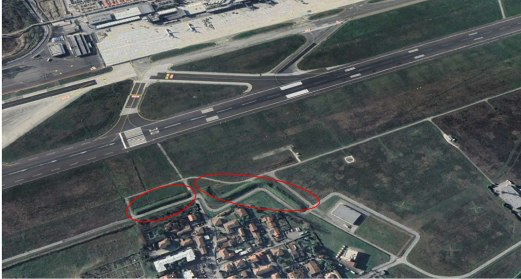
Figure 7: Noise barrier constructed by Bologna Marconi Airport to shield the Lippo residential settlement
