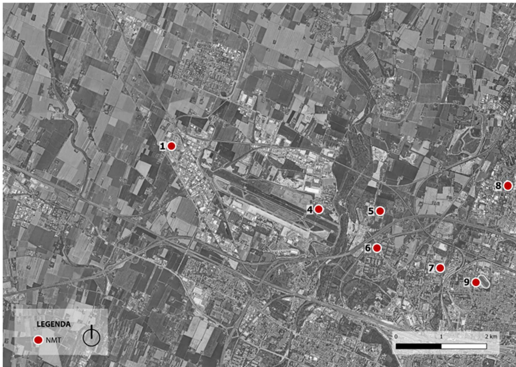
Figure 6: Noise Monitoring System at Bologna Airport
